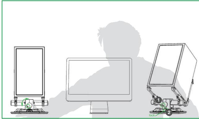
**Adjust your tilt with the tilt adjustment wheel ①. Position and lock your speaker with the rotate baseplate ②. Elevate Your Sound.**
